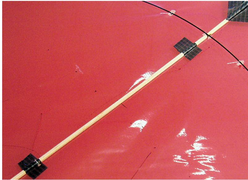
I decided to use a 3-point bridle, so I measured the location of the upper bridle connections; 2" either side of the spine center, and made a mark on the skin, then melted a hole there using my soldering iron. I make the hole reasonably large so the bridle doesn't get snagged on the skin during flight. And also for the 3-point bridle I melted a hole on either side of the spine at the lower bridle connection point as indicated on the template. All total, this took about 3 minutes.
