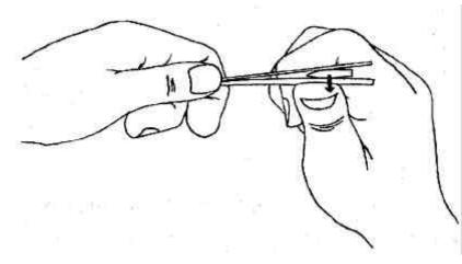
bamboo split. This may be useful if you're relatively new to working with bamboo. When the split is tending toward the top surface, as in the diagram, by pulling down with the knife, bending the lower split portion of the bamboo, the split will begin to move in the direction of the bend. This will direct the split more toward the center of the bamboo spine in the diagram. The reverse is true if you want the split to move toward the top.
