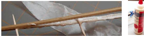
is a good tool for spreading the glue. I use glue by the name of 'WeldBond', it's waterproof white glue, but I think any waterproof wood glue or contact cement would work fine. I just happened to have some WeldBond so I used it. White glue remains slightly flexible after it dries, so the spine can be re-bent. If you use glue that is rigid when it dries the spine may not bend easily in the glued area after laminating. Choose the glue you think will work best for your desired result.
