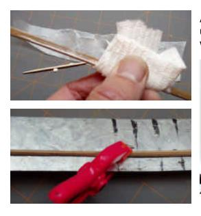
After applying the glue along the entire split surfaces, use a paper towel and bring the split parts together and wipe the excess glue from the spine. After the bamboo
