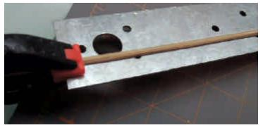
A NOTE ABOUT CLAMPS: One thing I noticed with clamps is that some have a strong enough spring to create a dent in the bamboo. The point were the dent is located is a weak point in the bamboo spine. Use clamps that will securely hold the two split parts together without denting the bamboo. That's why I use plastic clamps.
