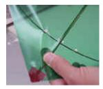
Using a small diameter soldering iron, touch the hot soldering iron to the kite sail at the dots on the lower part of the spine, at the points were the upper bridle connections are located on the bow. If you want to tie the bow and spine together, make holes for that at the crossing of the spine and bow. You could also
