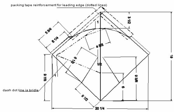
Bow 23 7/8" long. Use 0.05 carbon fiber for winds 0.5 - 5 mph. Use 0.06 carbon fiber for winds 3 - 9 mph.
