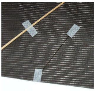
edge. Draw a straight line beginning at the trailing edge and extending 5" (127mm) toward the nose. Repeat for the other side of the kite. These lines are the locations for the kite's battens.
