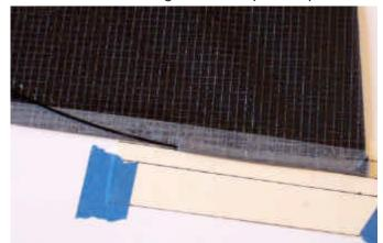
back side of the kite skin around the leading edge and bow. When folding it over the leading edge, where the bow is no longer at the edge, be careful not to bend the leading edge as you fold over the tape. Burnish it well. The tape bonds the bow to the kite skin.
