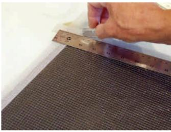
Carefully align the photo corner so the corner of the photo corner is on the corner of the kite skin's nose. The nose photo corner will actually be applied directly on the leading edge reinforcing tape. Press it down onto the nose of the kite on the reinforcing
