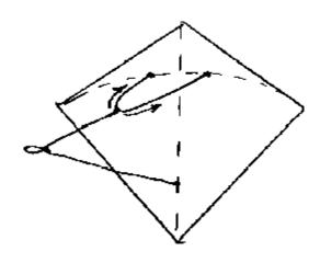
strong tension is applied to the flying line. When the right/left bridle adjustment is correctly positioned, the kite won't have any tendency to veer or constantly turn to one side or the other!
