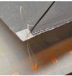
Measure ½"/6.35mm from the leading edge corner and make a mark on the leading edge. Do the same on the opposite leading edge corner.
