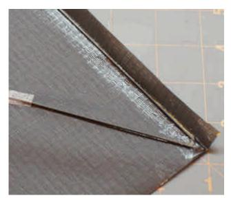
Once the glue is dry, fold the hem around the leading edge spar and onto the back side of the kite skin and burnish well.
