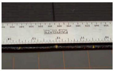
Thread a large eyed needle with about 12"/305mm of bridle line. Begin at one of the bridle marks you made on the leading edge and from the back side of the kite poke the needle thru the kite skin just below the leading edge spar. Pull the line through so there remains enough line to tie a secure knot. Then poke the needle from the front of the kite through the kite skin at the mark on the other side of the spine.
