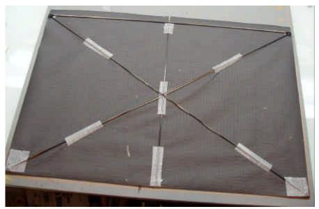
Burnish all the tape well so it is bonded well around the spars and also onto the kite skin. I use a toothpick to assist in the burnishing.
