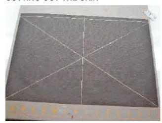
Measure a rectangle 10.5"/266.7mm x 15"/381mm on your skin material. This dimension includes a 1/2"/12.7mm hem along the leading edge that will encase the leading edge spar.
