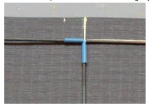
in alignment; it uses a small piece of tubing. You puncture one wall of the tubing with a needle at about the 1/2 length mark of the tubing. Then insert one end of the leading edge spar into one end of the tubing and have the spar exit through the puncture you made with the needle.
