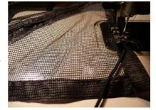
of molded deltoid) and frame the whole air inlet vent with some more stripes of nylon fabric.
