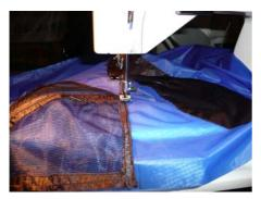
As soon as the back part is completed so far, you can sew the air inlet vent on the appropriate mark.
