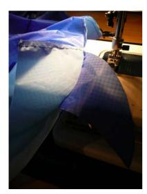
You are near the end of sewing and the back part can now be assembled to the side parts, start with the first side at the tip of the nose.
