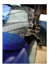
Do not fix the sides of the air inlet vent, because here are the air entrance and the valve flap.
