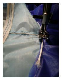
Stitch on a short piece of reinforcement line in the middle at point D. Later on here will be the attachment point for he drogue.
