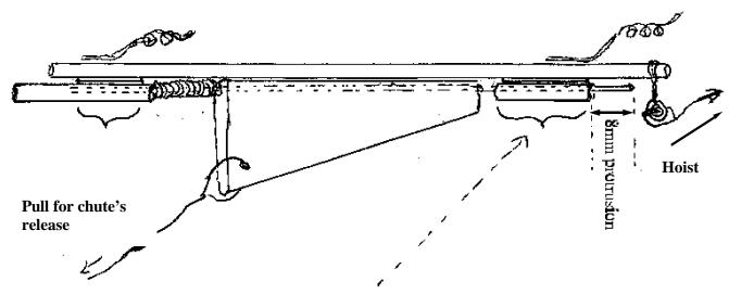
Where the inverted bracket is shown in sketch, use araldite and wind around tightly with thin wire (fuse wire will do), then wire wind to hold the launch bearers above the spine. When all dry add liberal coat of araldite to both strengthen the unit and make for least wind resistance. Do make sure to round off the top edge of the trigger, to ensure that should it rotate at all the corners will not foul the triggers action.
